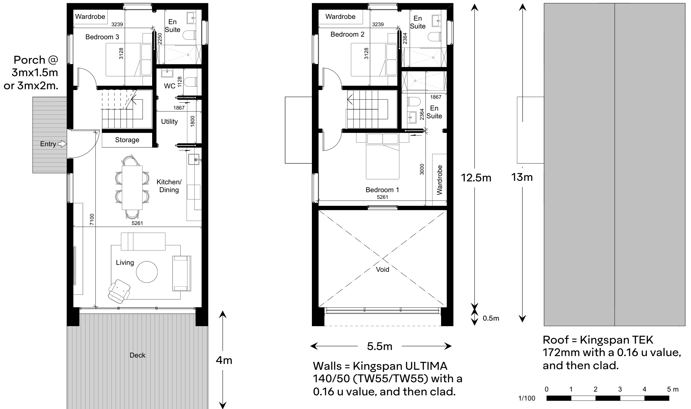
Figure 4. Floor plans & key dimensions.
